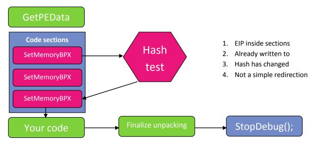
Figure (3) Generic unpacker algorithm layout
